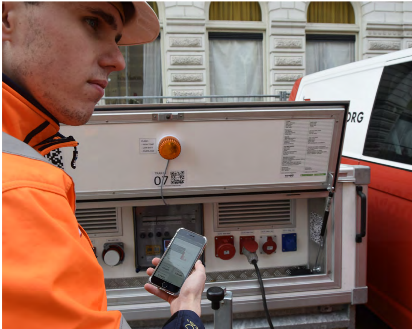
Some of our mobile tower cranes run a whole day on power using a battery cart or construction power.
