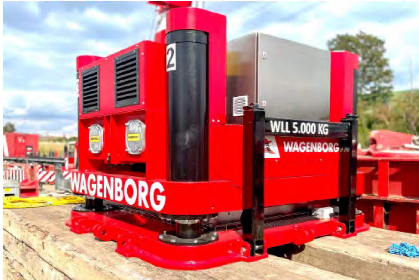
Enerpac jacking system
